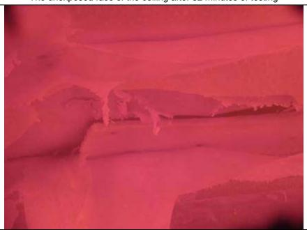
The exposed face of the floor assembly after 40 minutes of testing
