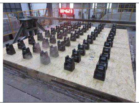
The unexposed face of the floor assembly after 46 minutes of testing
