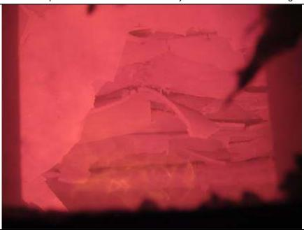
The exposed face of the floor assembly after 52 minutes of testing
