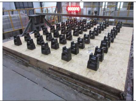
The unexposed face of the floor assembly before the test
